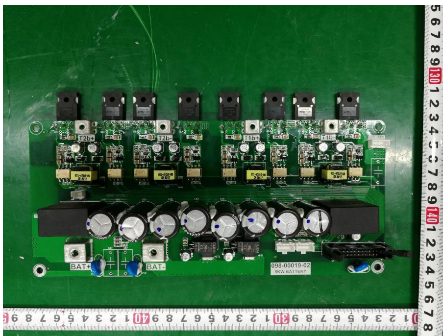
Component side of INV board
